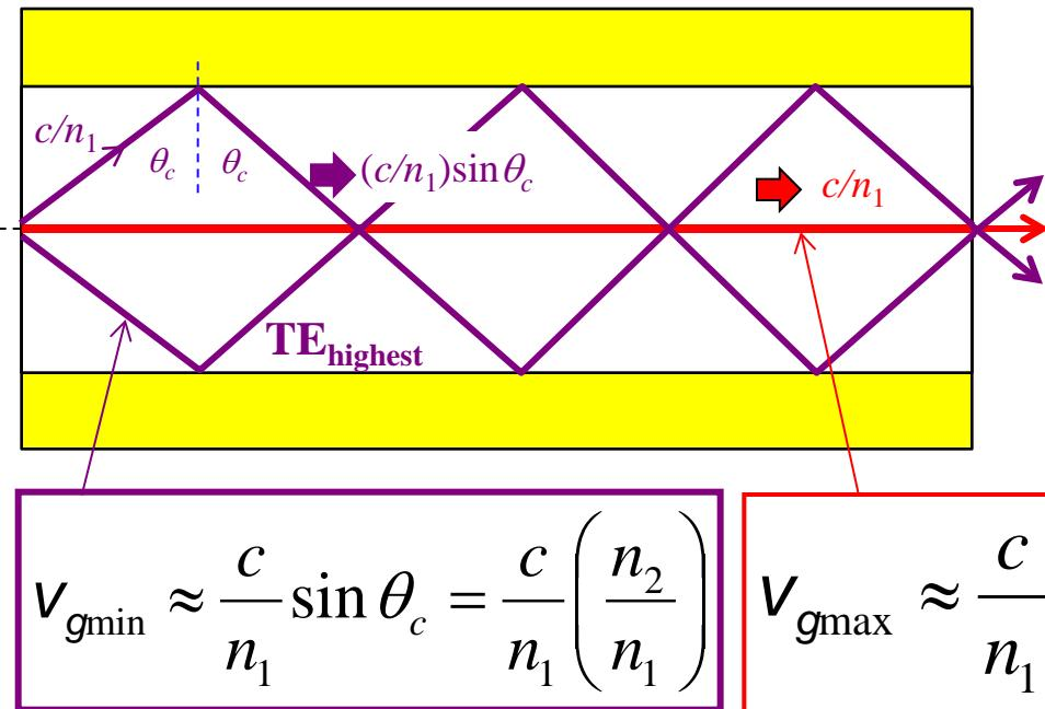
$$\frac{\Delta\tau}{L} = \frac{1}{V_{g\min}} - \frac{1}{V_{g\max}} \rightarrow \frac{\Delta\tau}{L} = \frac{n_1^2}{cn_2} - \frac{n_1}{c} = \frac{1}{c} \left[ \frac{(n_1 - n_2)n_1}{n_2} \right] \approx \frac{(n_1 - n_2)}{c}$$
