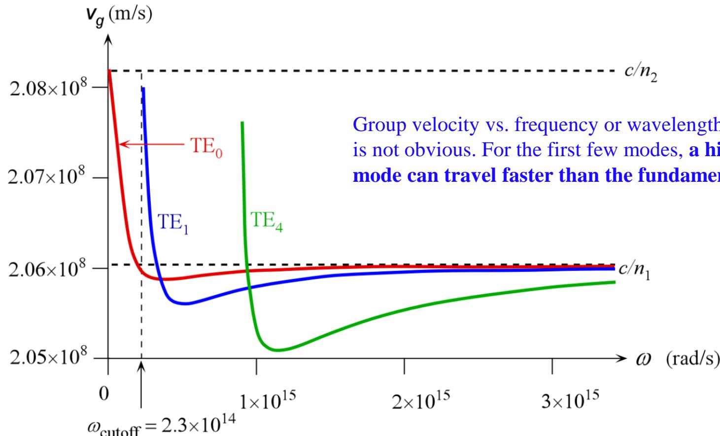
Group velocity vs. frequency or wavelength behavior is not obvious. For the first few modes, **a higher mode can travel faster than the fundamental.**
