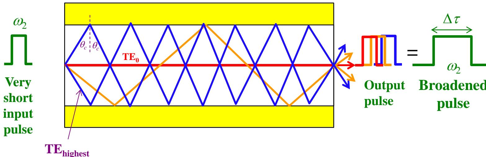
$$\frac{\Delta\tau}{L} = \frac{1}{v_{g\min}} - \frac{1}{v_{g\max}} \quad \rightarrow$$
