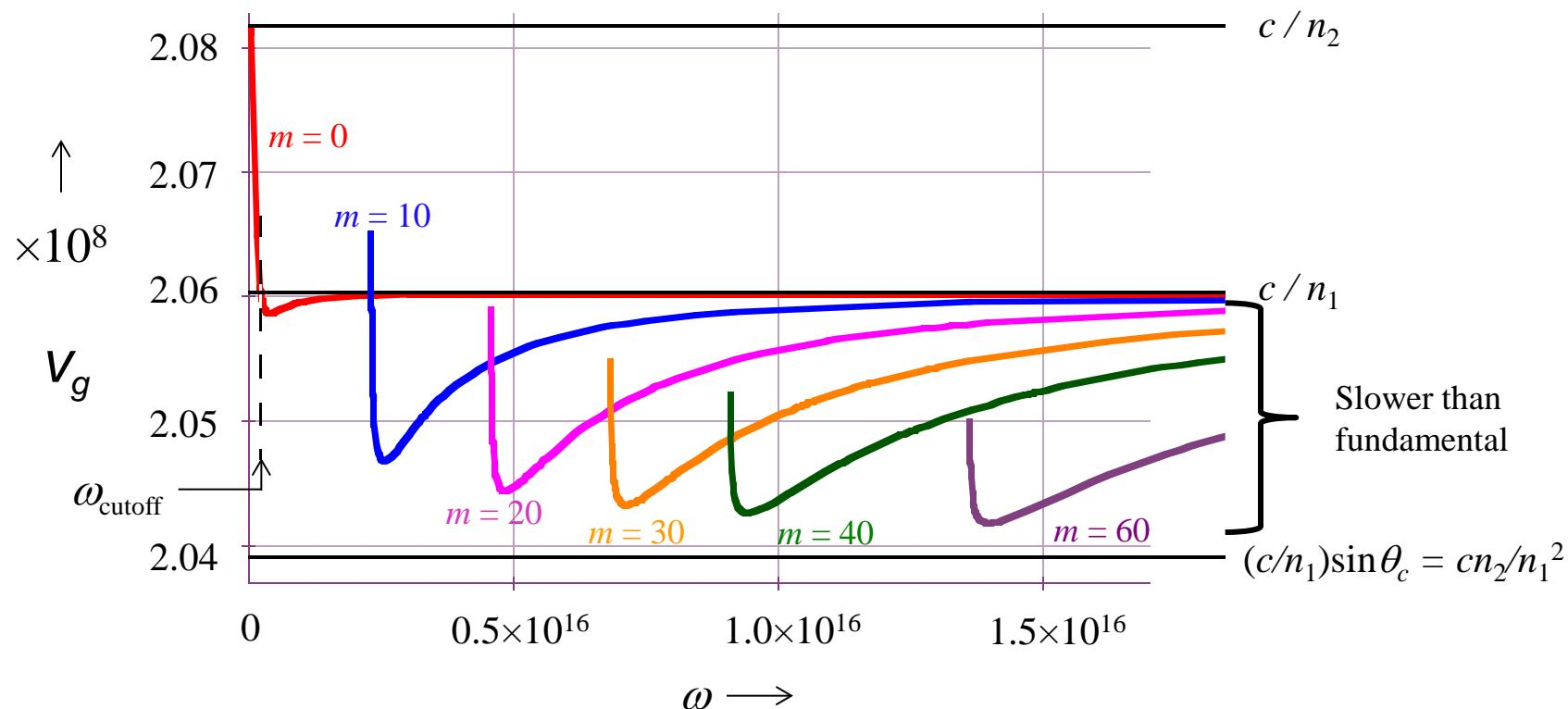
The group velocity  $v_g$  vs.  $\omega$  for a planar dielectric guide
