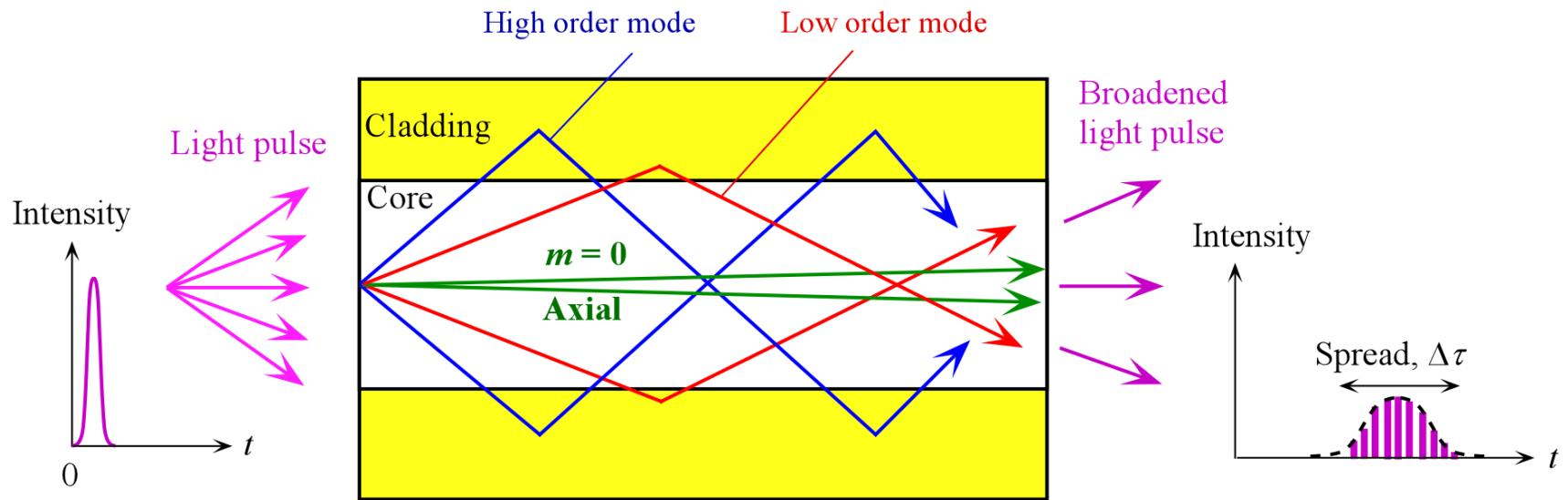
Schematic illustration of light propagation in a slab dielectric waveguide. Light pulse entering the waveguide breaks up into various modes which then propagate at different group velocities down the guide. At the end of the guide, the modes combine to constitute the output light pulse which is broader than the input light pulse.
