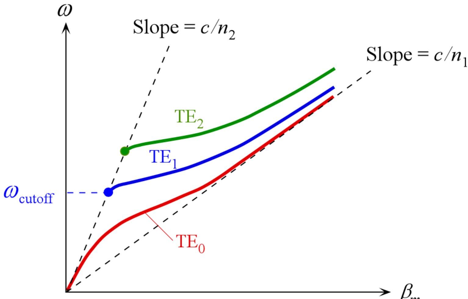
**The slope of  $\omega$  vs.  $\beta$  is the group velocity  $v_g$**
